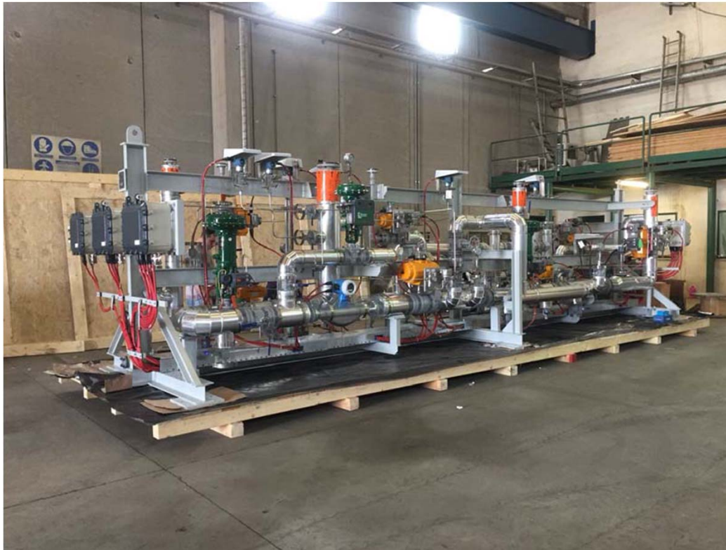
Firing skid, 4 inches 150#RF
